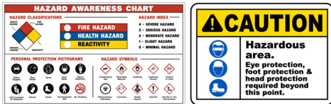
FIGURE 5: HAZARD SIGNS FOR COMMUNICATING RISK AND REQUIRED PPE ON SITE
